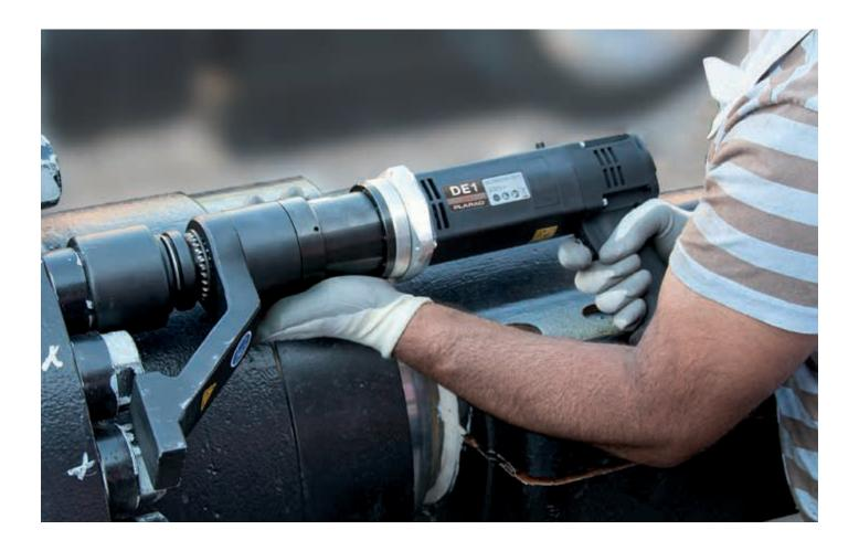
We have given the DE1 docu a new control system which includes voltage monitoring and speed sensing. This allows you to complete your bolting with even greater precision and reliability. As it reliably offsets any voltage fluctuations and changes in temperature, this new tool delivers superior torque accuracy. The DE1 docu switches automatically to the available mains frequency (e.g. 50 Hz or 60 Hz).
